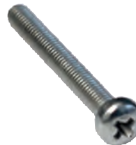
Fillister head screw · M 3 x 25 mm Part No.: 900-822-0049 Explanation: with slots and cross slots; only for valve system SF (for one valve system two screws are required); tightening torque max. 0,5 Nm
